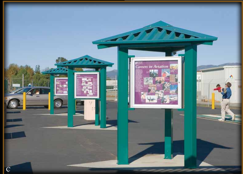
Observation Area at Van Nuys Airport, Van Nuys, CA: 7' Triangle Kiosk w/ 3' x 3' satin aluminum cabinets. 4:12 pitch HR-36 steel roof and frame are finished in Jade Green. Free flying lessons offered at right. Standard roof pitch is 6:12.
